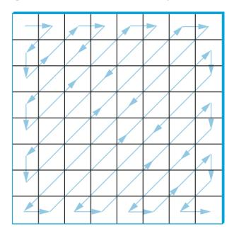
Figure 7.13.: Zigzag traversal of quantized frequency coefficients.
