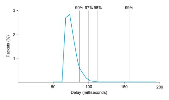
Figure 6.23.: Example distribution of delays for an Internet connection.
