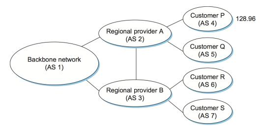
Figure 4.6.: Example of loop among autonomous systems.
