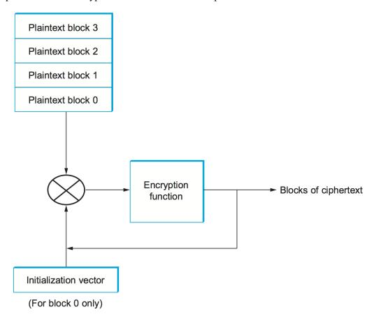
Figure 8.2.: Cipher Block Chaining.
