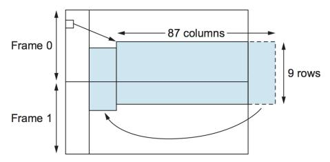
Figure 2.11.: SONET frames out of phase.
