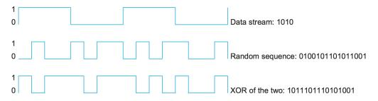
Figure 2.23.: Example 4-bit chipping sequence.
