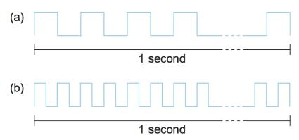
Figure 1.16.: Bits transmitted at a particular bandwidth can be regarded as having some width: (a) bits transmitted at 1 Mbps (each bit is 1 microsecond wide); (b) bits transmitted at 2 Mbps (each bit is 0.5 microseconds wide).
