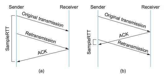
Figure 5.10.: Associating the ACK with (a) original transmission versus (b) retransmission.
