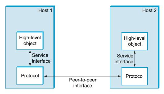
Figure 1.10.: Service interfaces and peer interfaces.
