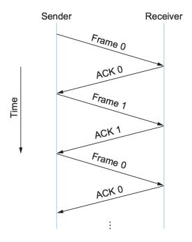
Figure 2.15.: Timeline for stop-and-wait with 1-bit sequence number.
