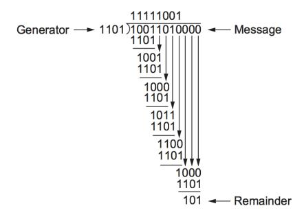
Figure 2.12.: CRC calculation using polynomial long division.
