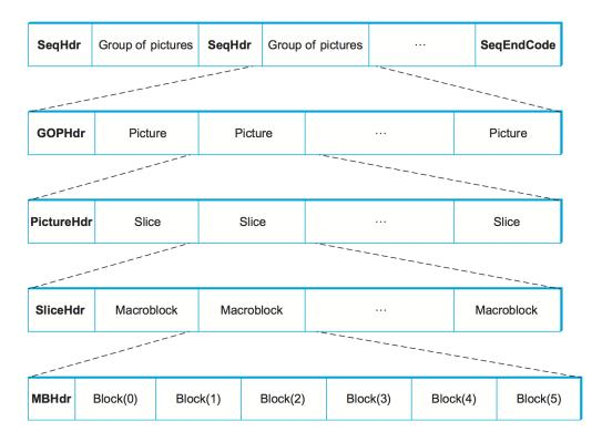
Figure 7.16.: Format of an MPEG-compressed video stream.
