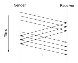
Figure 2.16.: Timeline for the sliding window algorithm.
