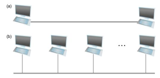
Figure 1.2.: Direct links: (a) point-to-point; (b) multiple-access.
