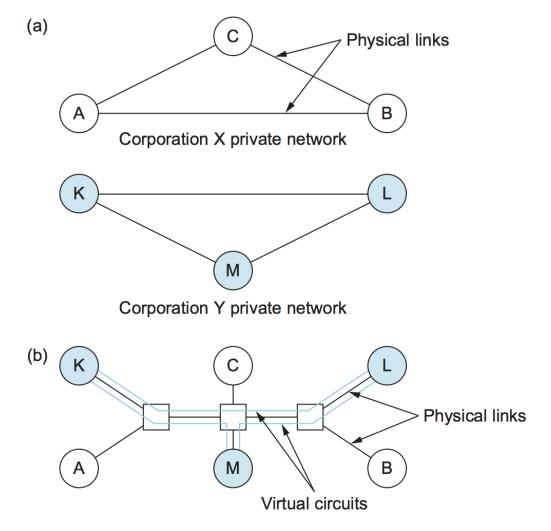
Figure 3.27.: An example of virtual private networks: (a) two separate private networks; (b) two virtual private networks sharing common switches.
