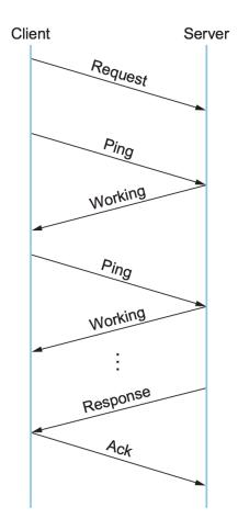
Figure 5.19.: Typical DCE-RPC message exchange.
