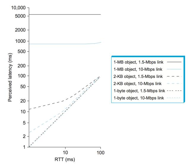
Figure 1.17.: Perceived latency (response time) versus round-trip time for various object sizes and link speeds.
