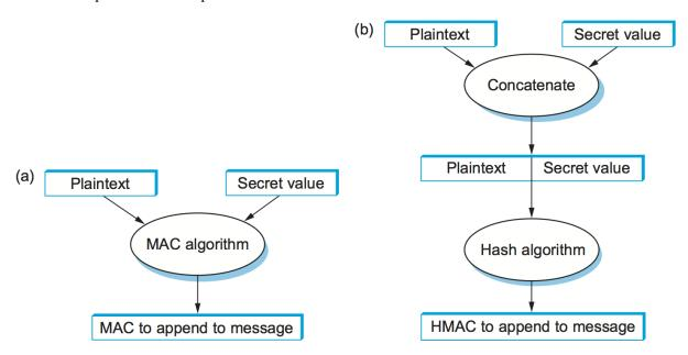
Figure 8.5.: Computing a MAC (a) versus computing an HMAC (b).
