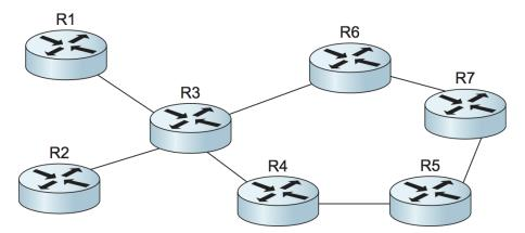
Figure 4.22.: A network requiring explicit routing.
