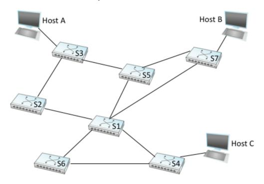
Figure 3.10.: Switched Ethernet with loops.
