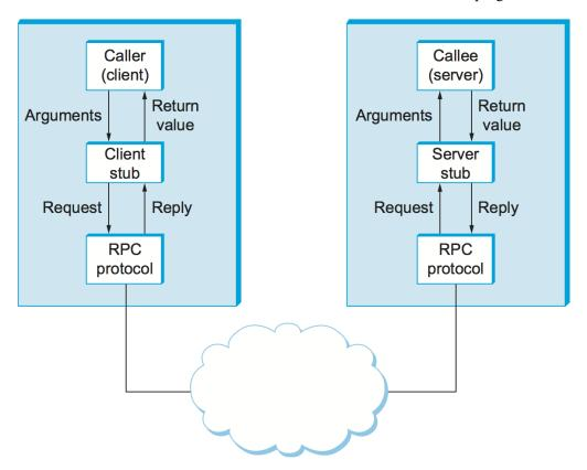
Figure 5.14.: Complete RPC mechanism.
