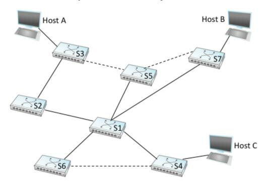
Figure 3.12.: Spanning tree with some ports not selected.
