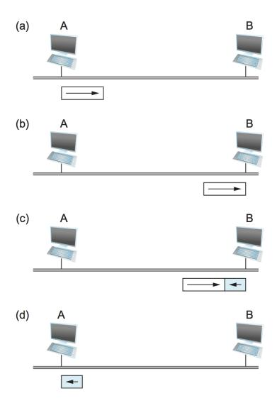
Figure 2.22.: Worst-case scenario: (a) A sends a frame at time t; (b) A's frame arrives at B at time t+d; (c) B begins transmitting at time t+d and collides with A's frame; (d) B's runt (32-bit) frame arrives at A at time  $t+2\times d$ .
