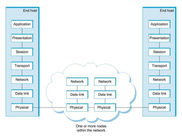
Figure 1.13.: The OSI 7-layer model.
