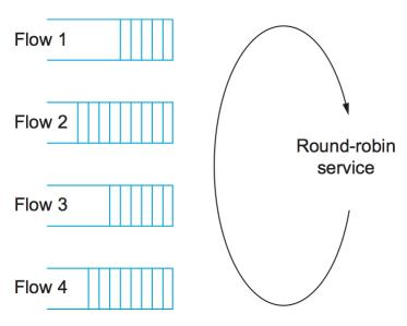
Figure 6.6.: Round-robin service of four flows at a router.
