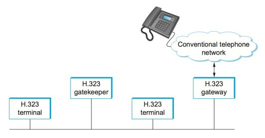
Figure 9.10.: Devices in an H.323 network.
