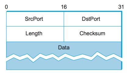
Figure 5.1.: Format for UDP header.
