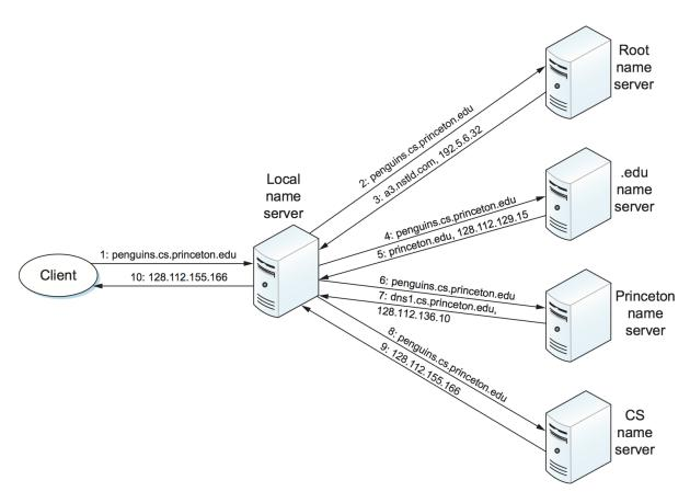
Figure 9.18.: Name resolution in practice, where the numbers 1 to 10 show the sequence of steps in the process.
