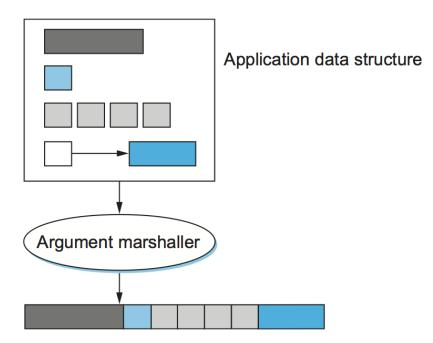
Figure 7.3.: Argument marshalling: converting, packing, and linearizing
