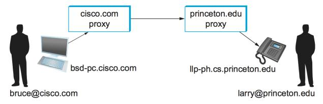
Figure 9.8.: Establishing communication through SIP proxies.
