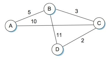
Figure 3.34.: Link-state routing: an example network.
