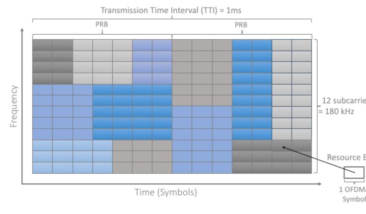
Figure 2.34.: The available radio spectrum abstractly represented by a 2-D grid of schedulable Resource Elements.
