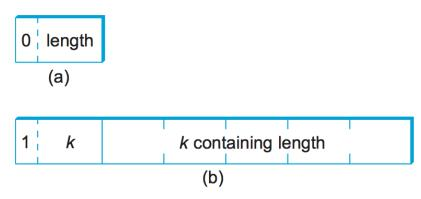
Figure 7.9.: ASN.1 BER representation for length: (a) 1 byte; (b) multibyte.
