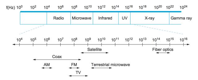
Figure 2.2.: Electromagnetic spectrum.
