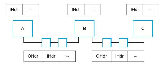
Figure 9.21.: Overlay nodes tunnel through physical nodes.
