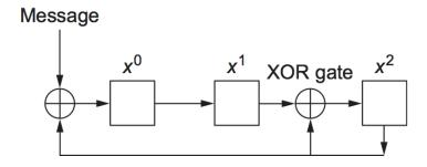
Figure 2.13.: CRC calculation using shift register.
