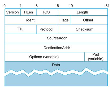
Figure 3.17.: IPv4 packet header.
