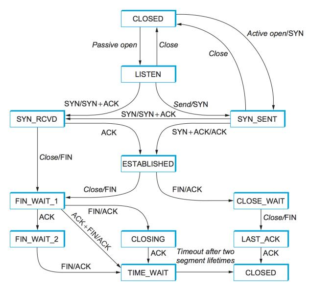
Figure 5.7.: TCP state-transition diagram.
