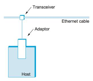
Figure 2.19.: Ethernet transceiver and adaptor.
