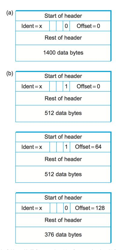
Figure 3.19.: Header fields used in IP fragmentation: (a) unfragmented packet; (b) fragmented packets.
