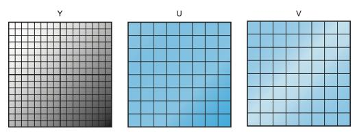
Figure 7.11.: Subsampling the U and V components of an image.
