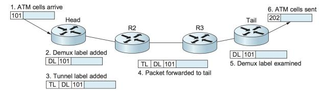
Figure 4.24.: Forward ATM cells along a tunnel.
