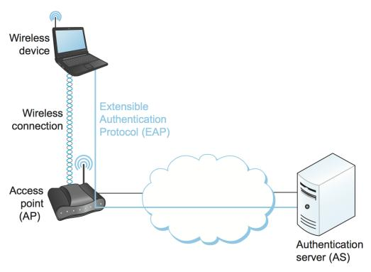
Figure 8.19.: Use of an Authentication Server in 802.11i.
