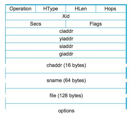
Figure 3.26.: DHCP packet format.
