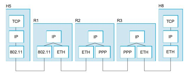
Figure 3.16.: A simple internetwork, showing the protocol layers used to connect H5 to H8 in the above figure. ETH is the protocol that runs over the Ethernet.
