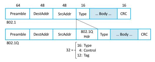
Figure 3.14.: 802.1Q VLAN tag embedded within an Ethernet (802.1) header.
