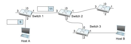
Figure 3.4.: A packet is sent into a virtual circuit network.
