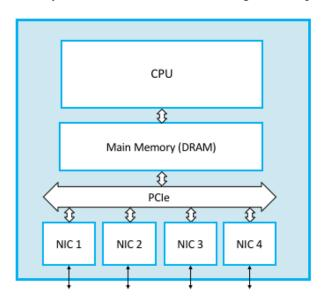
Figure 3.38.: A general-purpose processor used as a software switch.
