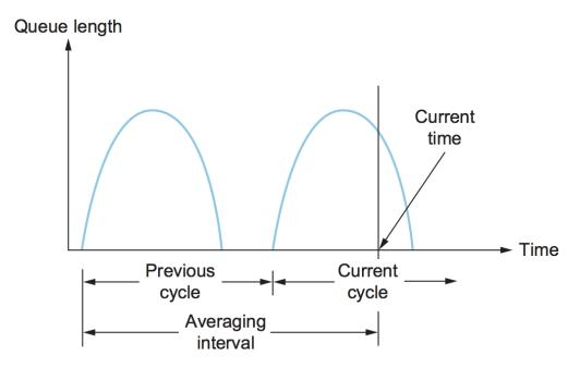
Figure 6.15.: Computing average queue length at a router.
