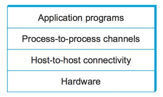
Figure 1.8.: Example of a layered network system.
