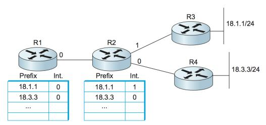
Figure 4.18.: Routing tables in example network.
