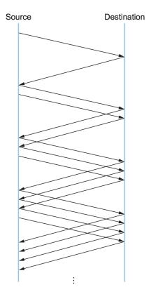
Figure 6.8.: Packets in transit during additive increase, with one packet being added each RTT.
