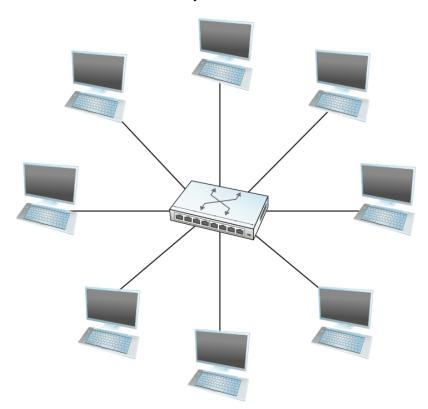
Figure 3.1.: A switch provides a star topology.
