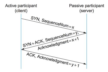
Figure 5.6.: Timeline for three-way handshake algorithm.
