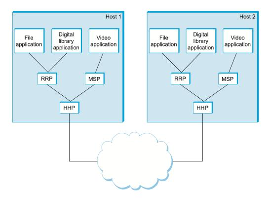
Figure 1.11.: Example of a protocol graph.
