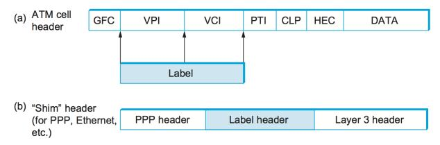
Figure 4.20.: (a) Label on an ATM-encapsulated packet; (b) label on a frame-encapsulated packet.
