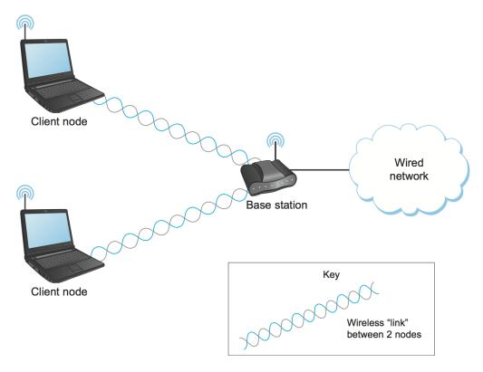
Figure 2.24.: A wireless network using a base station.
