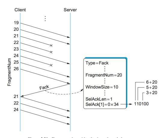
Figure 5.20.: Fragmentation with selective acknowledgments.
