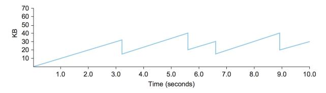
Figure 6.9.: Typical TCP sawtooth pattern.
