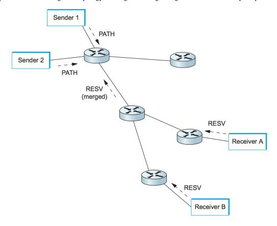
Figure 6.26.: Making reservations on a multicast tree.
