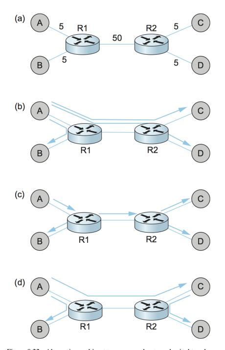
Figure 9.22.: Alternative multicast trees mapped onto a physical topology.
