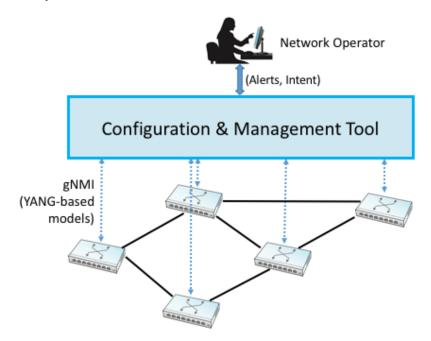
Figure 9.19.: Operator manages a network through a configuration and management tool, which in turn programmatically interacts with the underlying network devices (e.g., using gNMI as the transport protocol and YANG to specify the schema for the data being exchanged).
