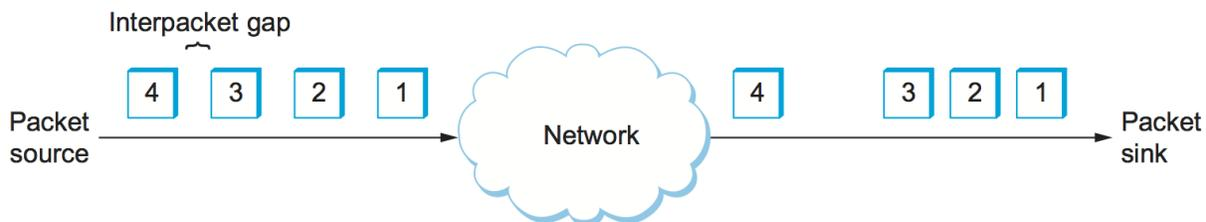
Figure 1.20.: Network-induced jitter.
