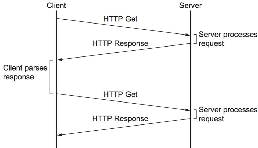
Figure 9.5.: HTTP 1.1 behavior with persistent connections.
