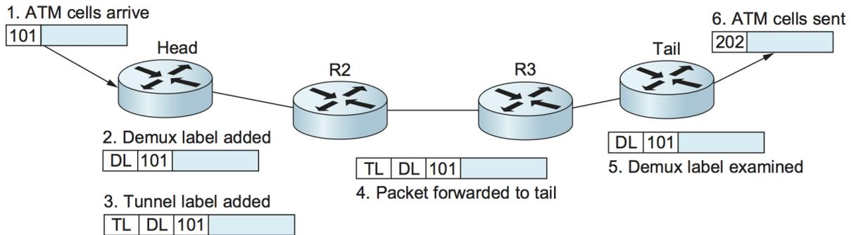
Figure 4.24.: Forward ATM cells along a tunnel.
