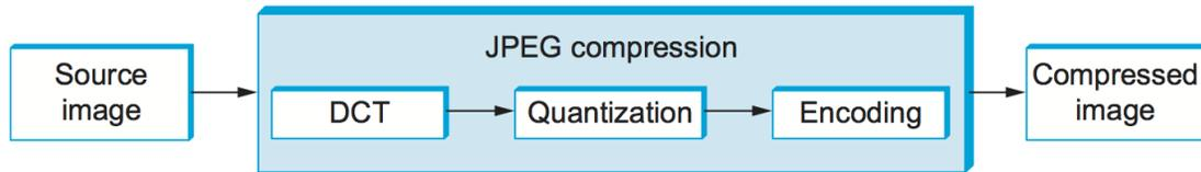
Figure 7.12.: Block diagram of JPEG compression.
