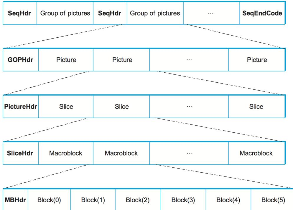
Figure 7.16.: Format of an MPEG-compressed video stream.
