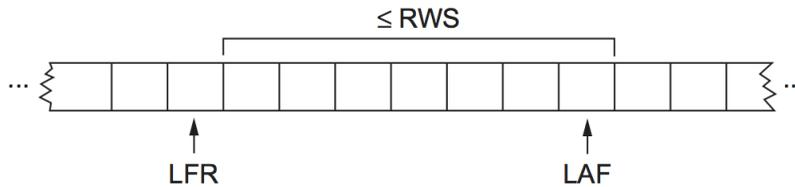
Figure 2.18.: Sliding window on receiver.
