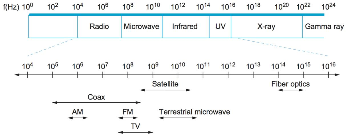
Figure 2.2.: Electromagnetic spectrum.
