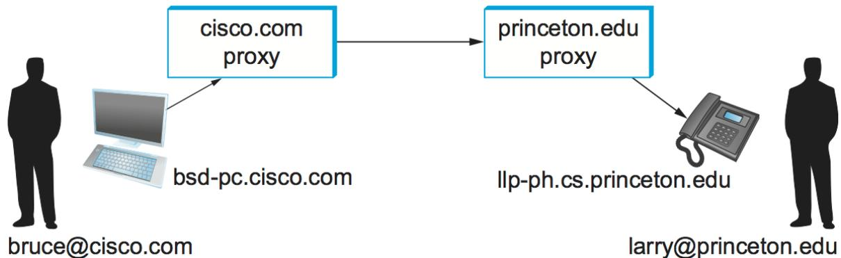
Figure 9.8.: Establishing communication through SIP proxies.
