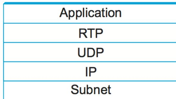
Figure 5.24.: Protocol stack for multimedia applications using RTP.
