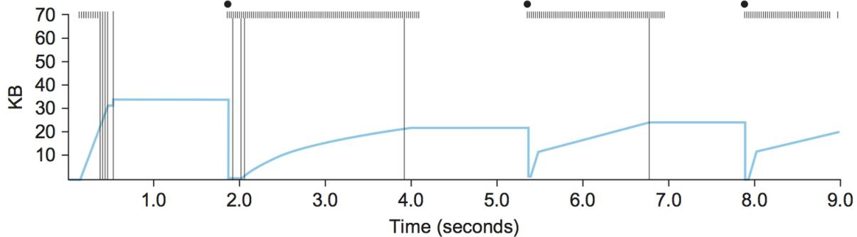
Figure 6.11.: Behavior of TCP congestion control. Colored line = value of `CongestionWindow` over time; solid bullets at top of graph = timeouts; hash marks at top of graph = time when each packet is transmitted; vertical bars = time when a packet that was eventually retransmitted was first transmitted.
