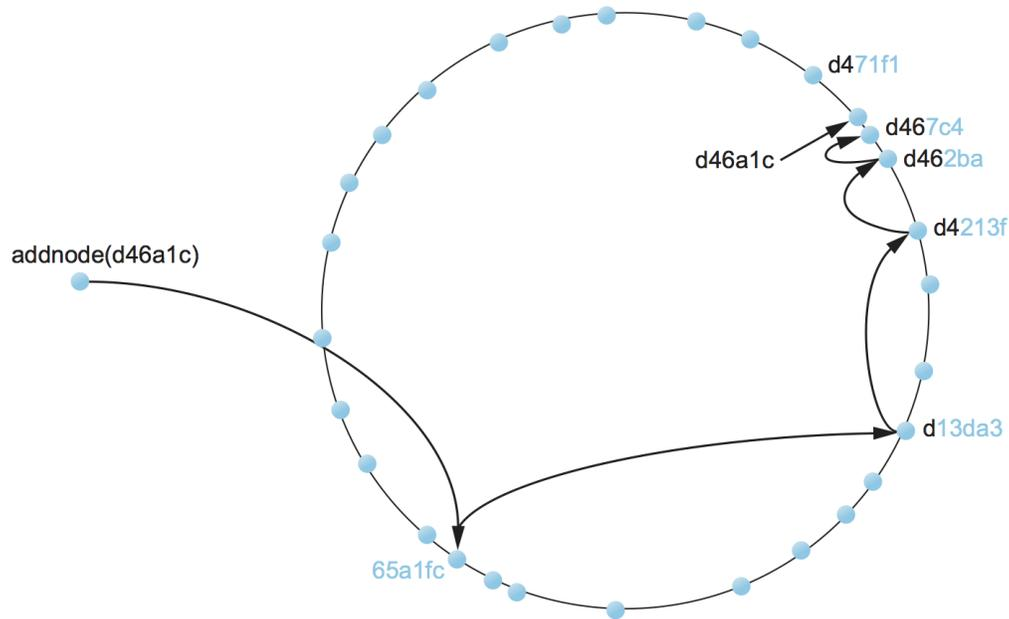
Figure 9.29.: Adding a node to the network.
