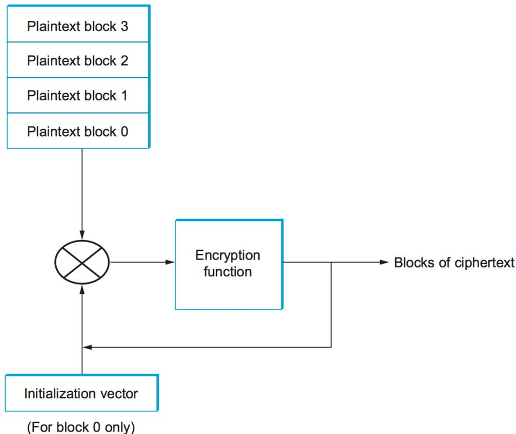
Figure 8.2.: Cipher Block Chaining.
